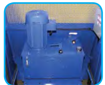
BE-QS Power Unit
